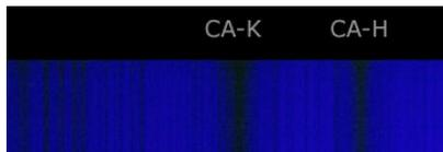
This distinctive part of the spectrum is also called CA-II. The K-line is very broad and can be split – with special, very expensive filters – into the components K1, K2 and K3. The Baader K-Line-filter has a half band width (HBW) of 8nm (80 Å). The human eye is almost blind at these UV-wavelengths, and at the same time UV-radiation below 390nm can cause severe damage to the eye. This is why the Baader K-Line filter is NOT approved for visual observation<sup>1</sup>.
