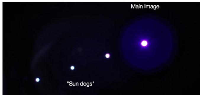
If you were to take a – very short – glance at the sun through the K-Line-filter in combination with Astro Solar Photo Film, you would see some asymmetrical, very dim “sun dogs” far away from the center of the image. They are caused by the tilt of the filters. With parallel filters, these reflections would all overlap and destroy the image quality. But since all reflections are directed to the side, you can image the centered UV-Sun through your telescope.
