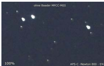
Picture detail at the edge to APS-C format with and without Baader MPCC
