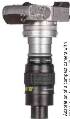
Adaptation of a compact camera with M43-thread to a Morpheus®-eyepiece
