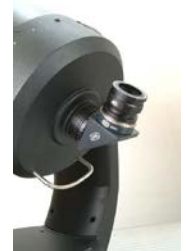
Celestron C8: BTA (#21), Maxbright star diagonal (#1A), T-2 quick changer (#6&7), ClickLock (#8)
