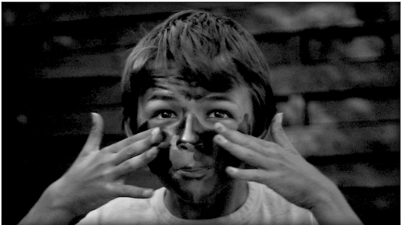
Suntan lotion in UV-A with Baader U-filter. It is invisible in visible light.
