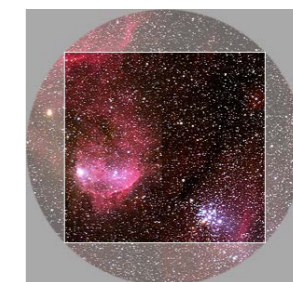
Usable field size of SBIG STX 16803 at 50mm flat field
