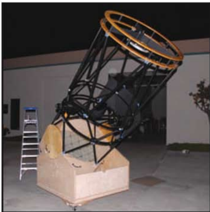
Image 2: First light for the CDK 42-inch Dobsonian telescope in front of PlaneWave Instruments.
