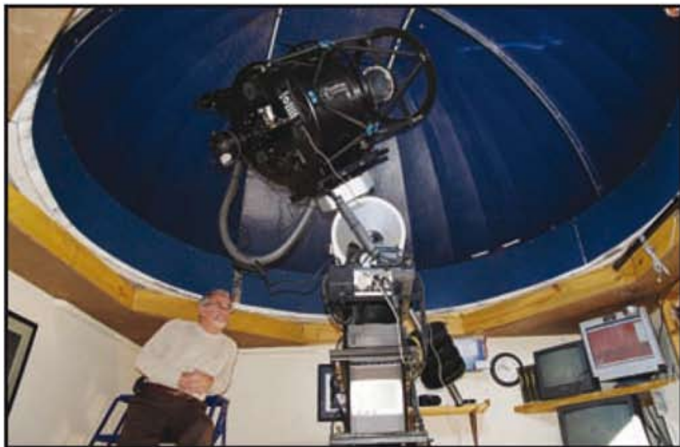
Dr. Clay Sherrod and the Arkansas Sky Observatories' Mathis Instruments MI500 mounted PlaneWave CDK17.
