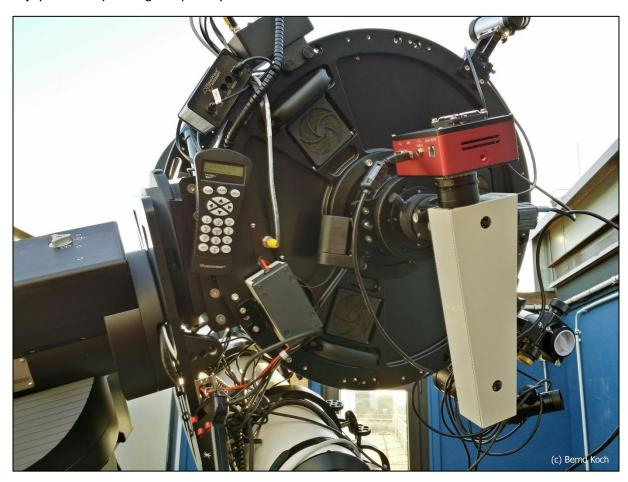
BACHES spectra are recorded with the STF-8300M CCD camera in 2x2-binning mode (effective pixel size  $10.8\mu m$ ). The monochrome Celestron Skyris 274M video camera serves as a guider camera. The Remote Calibration Unit (RCU) is located in the adjacent control room next to the right monitor and is controlled by PC. From there, the light from the Thorium-Argon/Halogen calibration lamps is conducted to the BACHES via a fiber cable.
