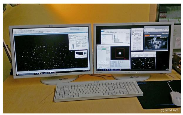
The desktop of one of the two monitors is duplicated on the monitor in the observation room. If you stand next to the telescope, you can do all settings in the observation room by mouse and keyboard before you enter the control room. This is particularly useful for observations directly at the telescope.
