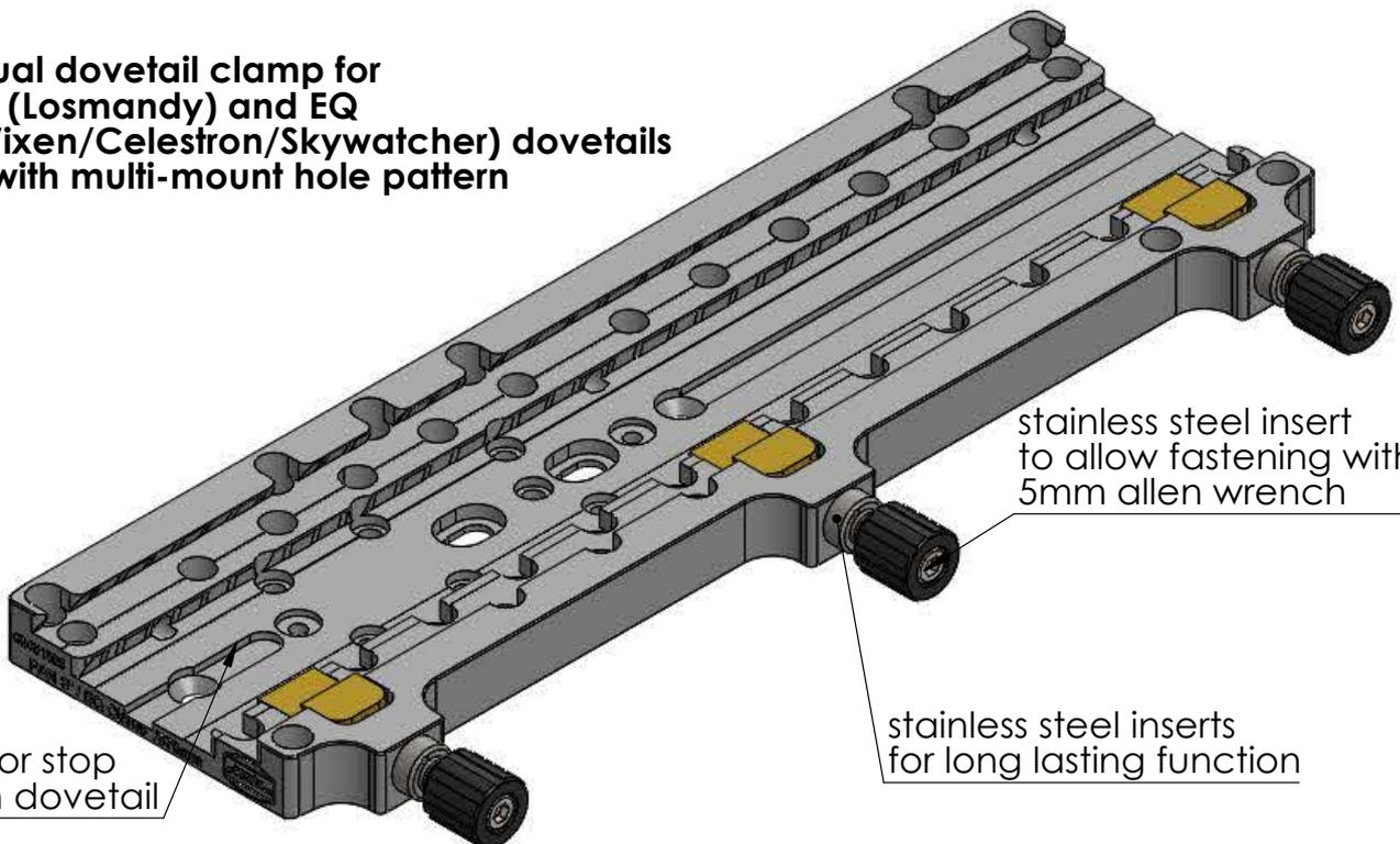
stainless steel insert to allow fastening with 5mm allen wrench
