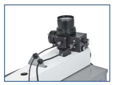
Attach the fiber to the fiber coupler. Take care to not scratch the polished front window of the fiber while plugging it in.
