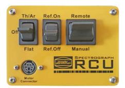
Shift the right switch to **Remote** to enable remote control
