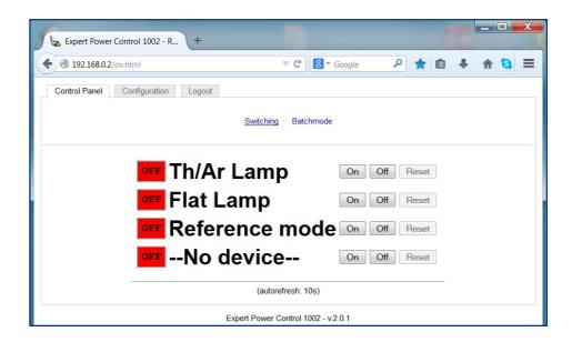
You can switch the RCU ON and OFF simply by typing the buttons of the LOGIN window. Then you can simply switch the devices ON and OFF as shown above.
