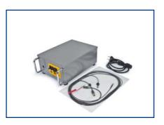
Attach the fiber and the power cord to the **front connectors** of the RCU. Do not try to plug on the RS232 socket at the rear side of the RCU. You are now ready to start working with the RCU.
