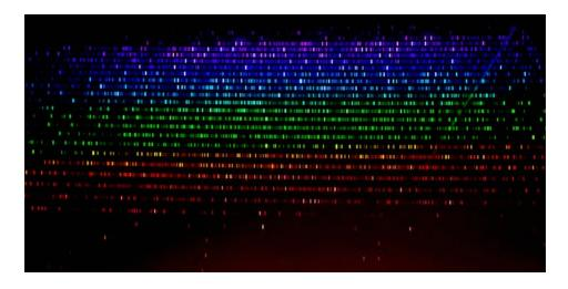
Thorium-Argon spectrum obtained with a Nikon D7100 DSLR camera, exposure time 10s at ISO 1000
