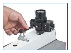
Gently fasten the fiber coupler to BACHES head using the supplied screws. The fiber coupler may need some alignment to work properly; how to do that is explained later on in this manual.
