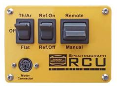
Switch to the **Th/Ar** lamp. The integration time for Th/Ar is usually a little shorter then for the flat-field lamp.
