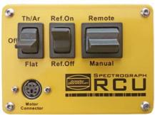
Shift the left switch to **Flat** to enable the flat-field lamp. Attach an eyepiece or camera to BACHES per its instructions manual.
