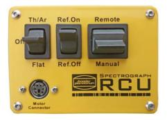
Shift the right switch to **Manual** and the middle switch to **Ref. On**. This will flip the coupling mirror in the BACHES head into the calibration position. For accurate calibration, ONLY calibration lamp light may illuminate the BACHES'
