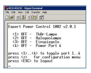
If the connection is successful, the RCU replies with a login screen. Now the power ports can be switched ON and OFF by typed commands from the PC. An explanation of available commands will be shown as well.
