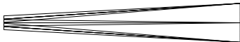
Light path of a 6" refracting telescope, which is expanded to f/30 with a Barlow lens (light coming from the left).
