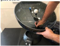
5. Unscrew the cap nut (made of metal or plastic depending on the year of manufacture):
