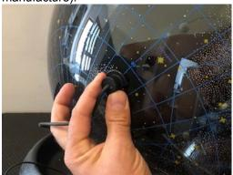
6. The cap nut with the slotted ring will slide down along the cable:
