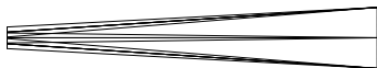
Light beam of a 6" lens telescope, which was extended to f/30 with a barlow lens
