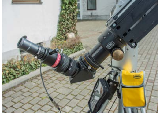
SunDancer II at a telescope with mirror star diagonal. Hand control and power supply are stored in the yellow bag.
