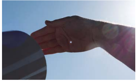
The concentrated, reflected solar radiation in front of an 80 mm telescope without D-ERF in front of the objective.
