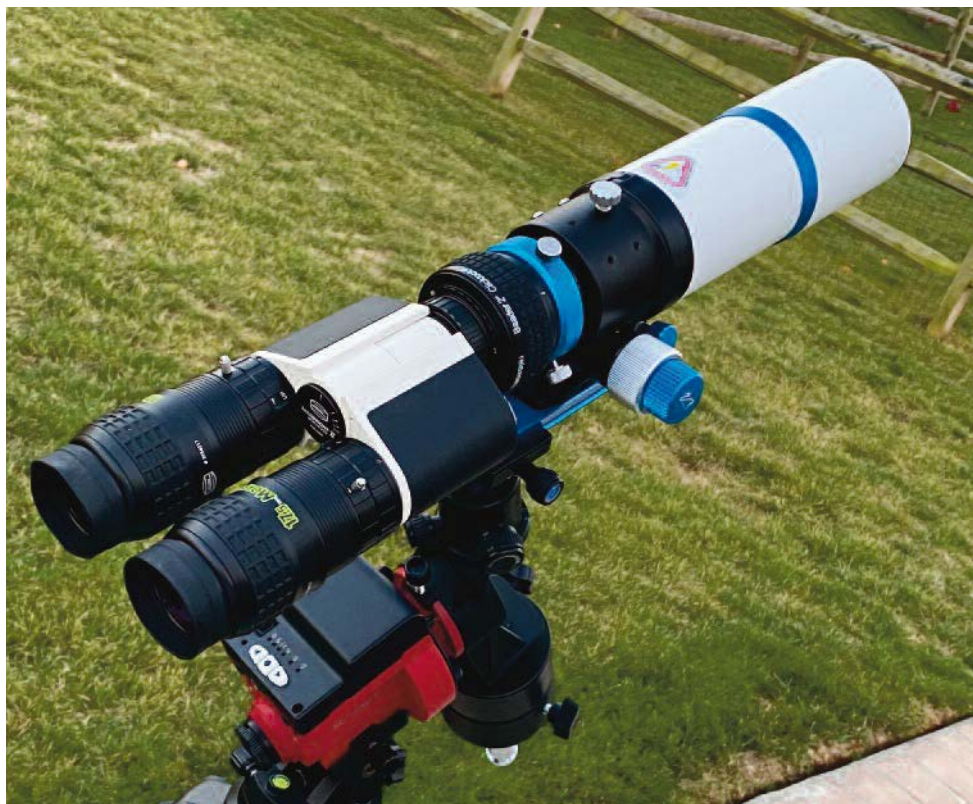
Image 1 – Binoviewer setup on my SkyGuider Pro – William Optics ZenithStar 61
