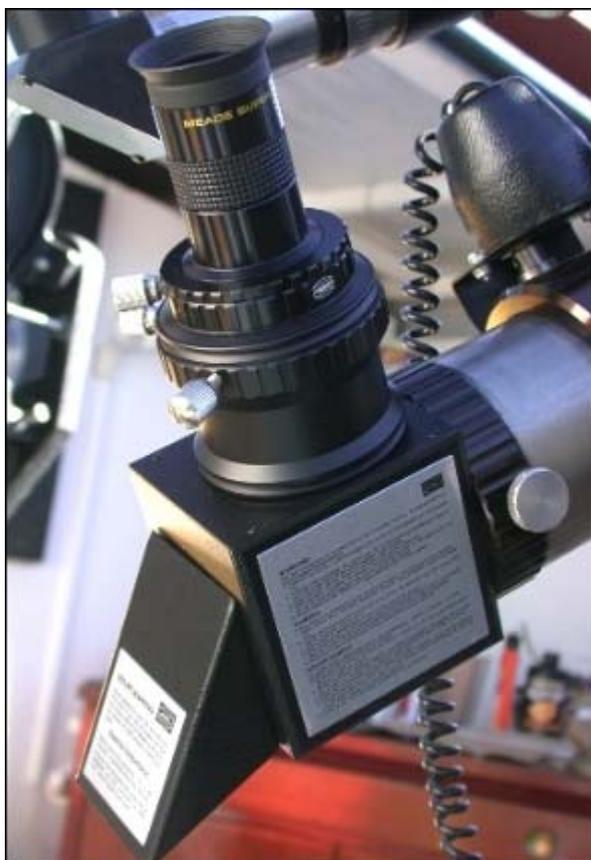
1. Without pointing the scope at the Sun connect the Herschel to the telescope, making sure that the ND-3 is screwed in place.
