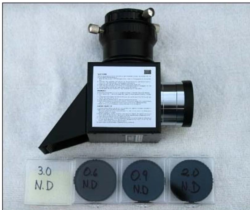
1. A very nicely made almost cubic housing that contains the Herschel prism, built of metal and beautifully crafted, sporting a shroud opposite to the 2" outside diameter chromed plated tube that connects to the telescope.
