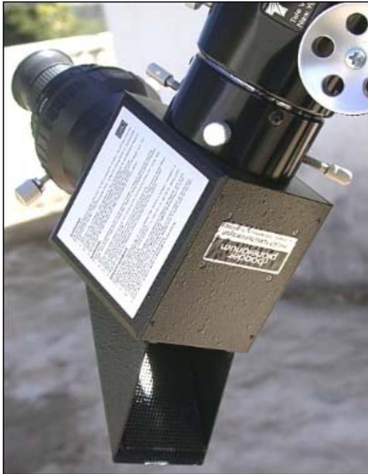
Here Baader has come with an elegant and simple solution, no more light and heat out the backdoor, ¿how? With a “Light trap” that Baader designed, I have tried it and believe me no heat and no light reflected to harm or burn out of the housing. That finishes with the fire hazard and related problems that plague the Herschel wedge, you can even glimpse inside the exhaust port and you see nothing that can harm you.
