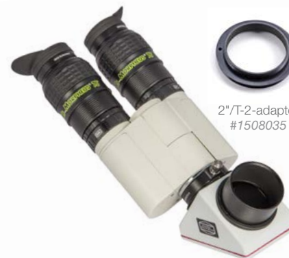
Short and sturdy adaptation e.g. of the Mark V binoviewer with the 2"/T-2-adapter #1508035 directly behind a 2" star diagonal.
