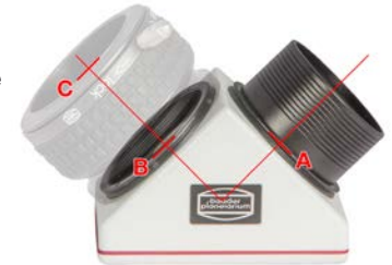
The required backfocus can be reduced from 112 mm with ClickLock® (A-C) to ca. 71,5 mm without ClickLock® (A-B).
