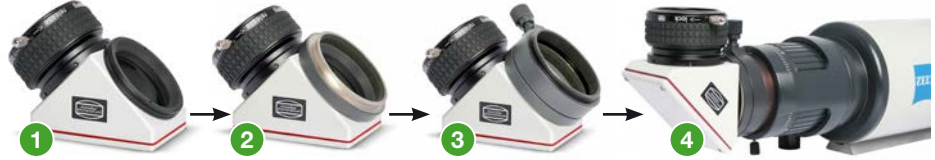
Connecting the M68 star diagonal: 1 The M68-thread 2 The attached M68/S68 Zeiss Changer #2458180 3 The S68/M68-Zeiss-Quick Changer added #2458185 4 Attached to a Zeiss APQ telescope. With the adapter #2458234, the ClickLock® on the eyepiece side can also be replaced by a M68-Quick-Changer.
