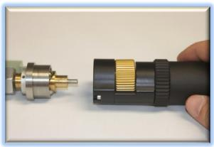
Use a gentle back and forth motion to slide the motor assembly on the shaft and then locate the clamp onto the stainless housing.
