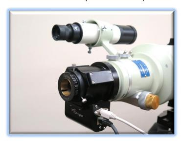
temperature response for any telescope is the tube. As aluminum and even carbon fiber tubes cool down they tend to shrink causing the focus to shift.
