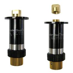
Unthread the brass stop from the end of the MicroFocuser. This stop prevents the telescope mirror from falling off the baffle tube inside the telescope. Thread the stop onto the focus shaft of the telescope. Be sure to thread the stop on far enough that the end of the threaded rod is exposed.
