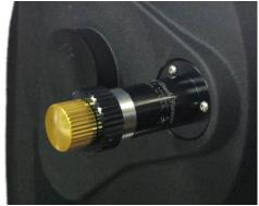
Use the three provided hex-head screws and wrench to attach the SCT MicroFocuser to the telescope. You are now ready to head out under the stars! Use the black knob for coarse focus and the brass knob for fine focus (10:1 ratio). Note that the telescope will likely be pretty far out of focus, so you may need to turn the focus knob quite a few times to reach focus.
