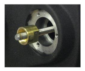
Snap the C-clip back onto the end of the threaded rod or thread the screw back in. Note that the C-clip fits into a small groove about 3 threads in from the very tip of the threaded rod. If your scope has a washer and screw, put these back in place on the focus shaft.
