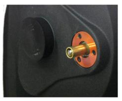
Begin by removing the black rubber focus knob from the scope. This knob simply pulls off the brass focus cylinder.
