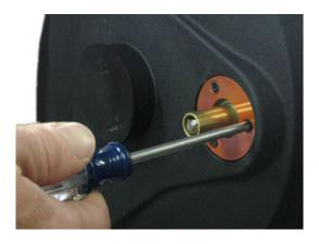
There are 3 small Phillips-head screws which hold the orange focus assembly cover in place. Remove these screws and take off the flat cover plate, exposing the inside of the focus assembly.
