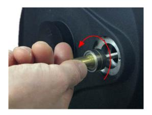
Rotate the brass portion of the focus shaft *counterclockwise*. This will unthread the brass cylinder and bearing assembly from the threaded rod. Remove these parts entirely (you will have to turn the brass shaft quite a few times to remove it).
