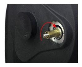
Rotate the brass portion of the focus assembly *clockwise*. This will bring the mirror back and expose the threaded portion of the focus shaft. At the tip of this threaded bolt will be either a small C-clip or a Philips-head screw and washer which will be removed in the next step.
