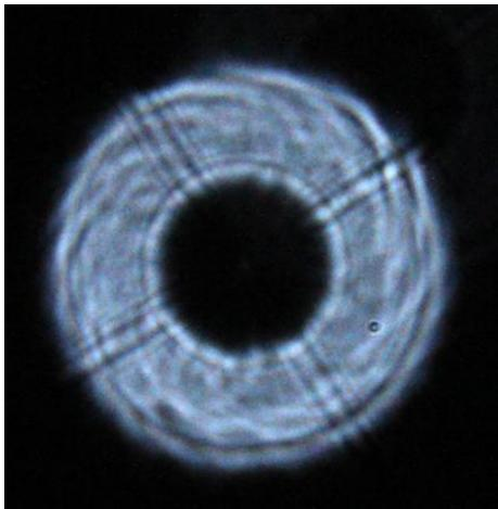
**The first surprise** at first light of the visual image at a magnification of about 150x with medium seeing conditions was that the unsharp star image appeared completely round with the dark shadow of the secondary mirror well centered. This means that after a UPS transport over 600km from Bavaria to Lower Saxony the collimation of the secondary mirror adjustment has been preserved. The picture left shows the defocused star disc **WITHOUT** any readjustment.
