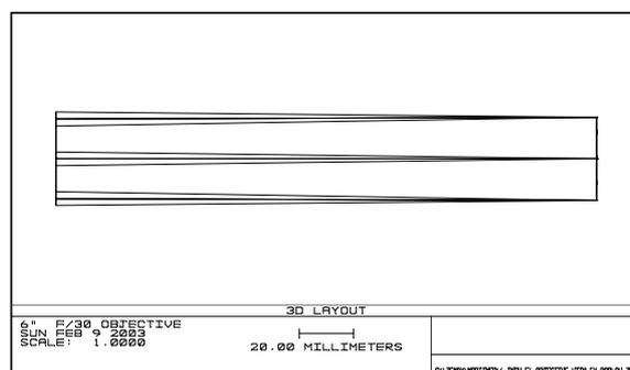
*This ray trace shows an f/30 telecentric design. The rays are uniform across the image plane. This does not mean that they are all going through the filter perpendicular to the image plane but the rays are parallel to the central rays.*
