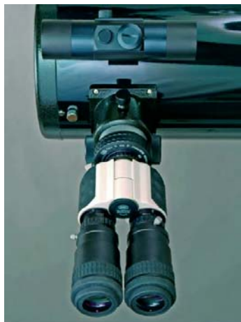
Maxbright-Bino am 8" Newton, - 2" Four-in-One-Adapter, 2" Newton-Komakorrektor 1.7x, 5 mm Hyperion-Okulare, Baader Skysurfer V Visiersucher
