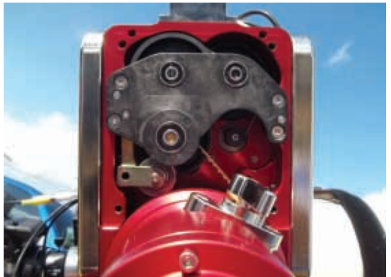
Image 4 - The M-Uno's "Fast Reverse" drive: a tooth belt-pulley system.
