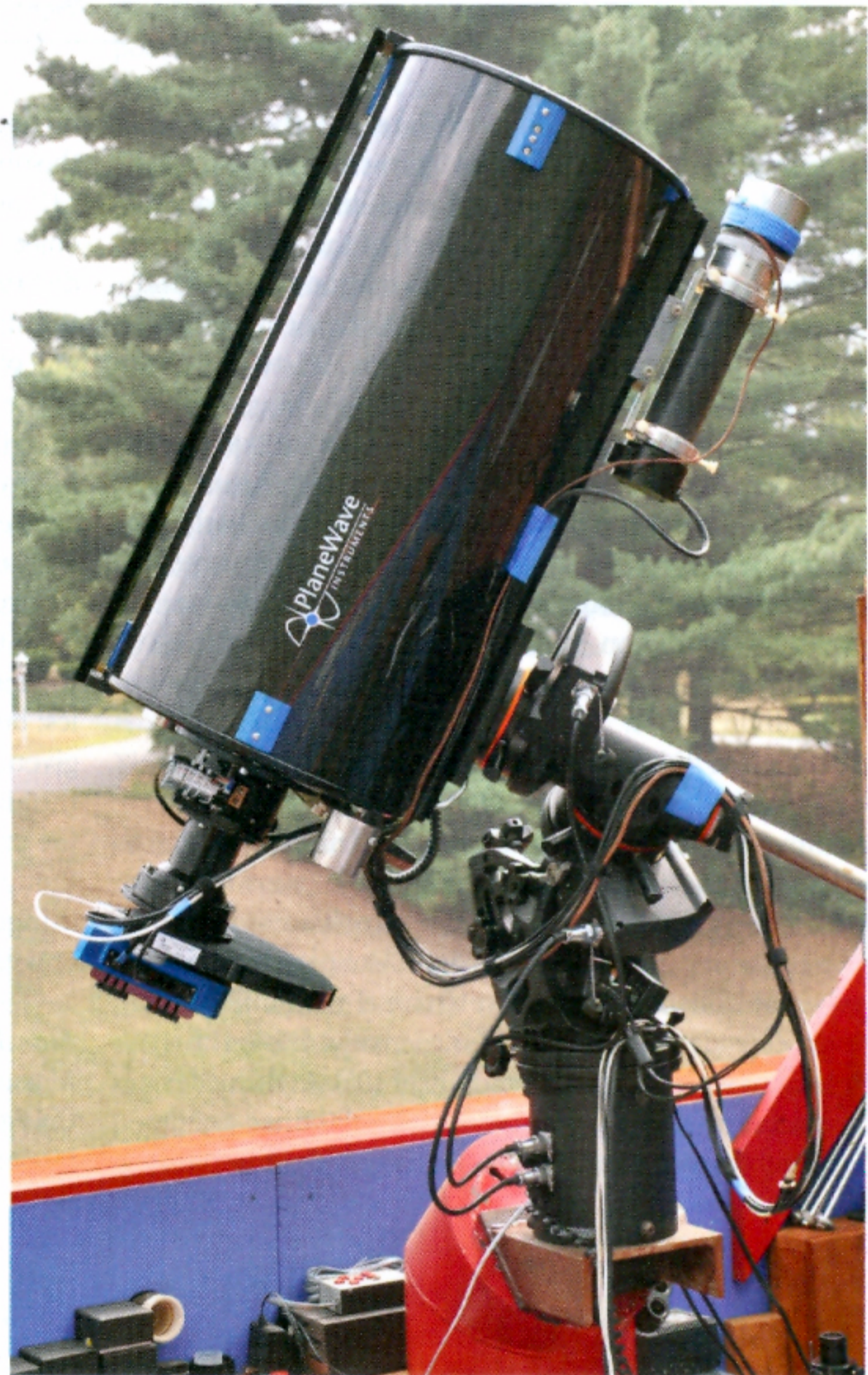
Pictured as tested in the author's suburban-Boston backyard observatory, the PlaneWave 12.5-inch f/8 CDK reflector was designed from the get-go as an astrograph for high-end CCD cameras. Little niceties such as 1/4-20 bolt holes in the tube's back plate and front ring make it easy to attach counterweights and other accessories used by astrophotographers.
