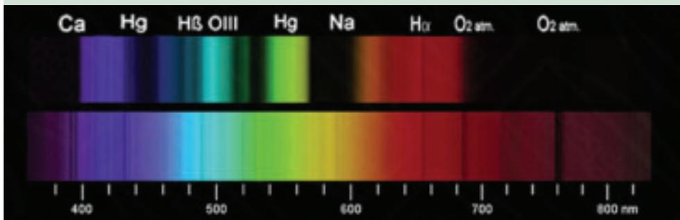
Image 3 - Spectrum of the Baader Neodymium Moon & Skyglow filter above the solar spectrum.
