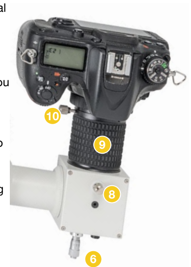
The necessary parts for focusing a camera and selecting the wavelength range, shown here with a DSLR
