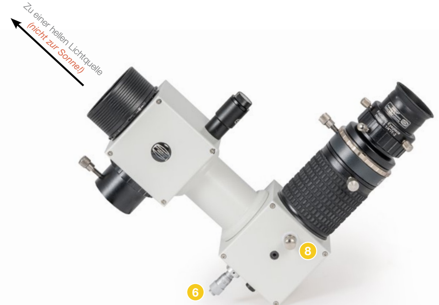
Setting the spectral range with the mikrometer 6 after loosening the locking screw 8
