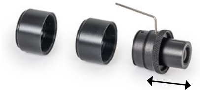
Remove both extension tubes to access the lens cell. Use the Allen wrench to unlock the lens cell and to slide it in or out.
