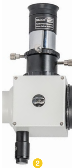
The micrometer for adjusting the slit illumination.
