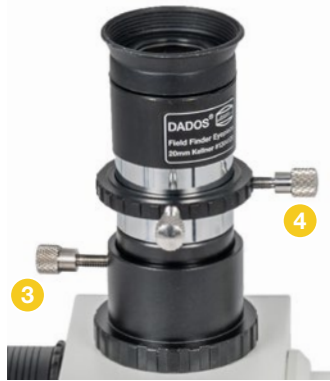
Move the eyepiece up and down, until you can see the three slits sharp, then lock it in place.
