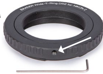
The inner thread of a T-2 ring (shown here: Baader Wide-T-Ring for Nikon Z #2408335) can be rotated into a convenient position by loosening three small setting screws.
