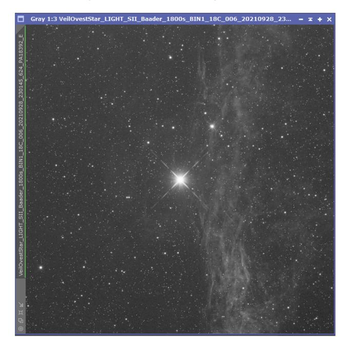
The average FWHM value is 1.80 arc seconds, very good and in line with expectations, considering the wavelength of the passband. Sky background measured in about 620 ADU, also in this case the gradient is very low, similar to the result of the H-alpha filter, with a delta of about 30 ADU. The diffraction figure of the main star is in line with the other two filters, but in this case the visibility of the reflection on the deflecting glass of the active
