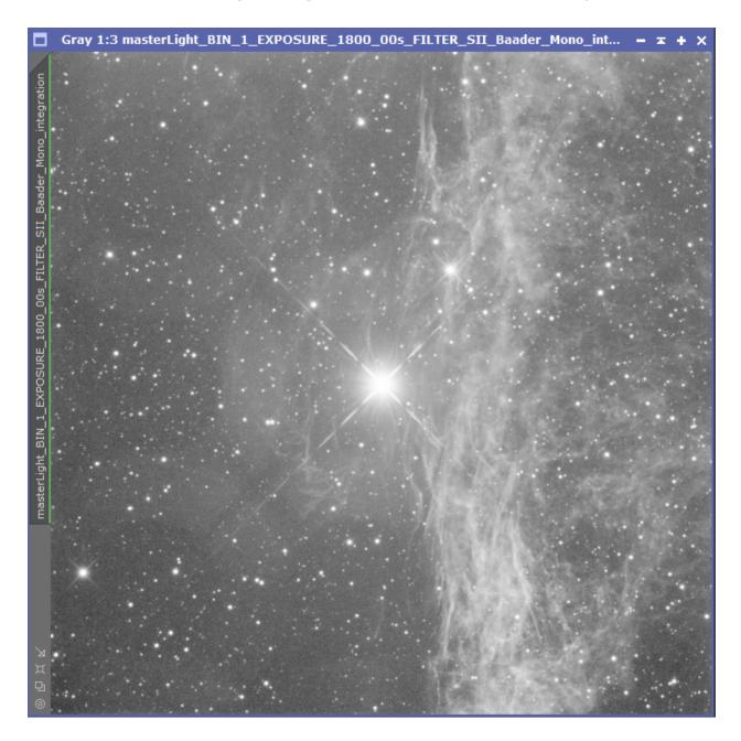
The structures of the primary reflex and secondary reflexes are visible over the whole field. Comparative tests with the inversion of the filter itself and with another identical Baader Ultra Narrowband SII filter, tested later, confirm the result. Further comparative tests were carried out on a filter of another well-known European brand, with a passband of 12nm and produced a slightly worse result, confirming the criticality of the specific optical train,
