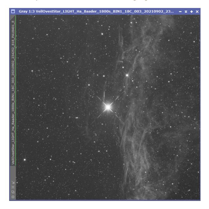
The result in terms of stellar diameter is in my opinion very good, measured in an average FWHM of 2.07 arc seconds. The narrow passband guarantees the absence of gradients (delta about 30 ADU) with a sky background of only 630 ADU and well-engraved micro
