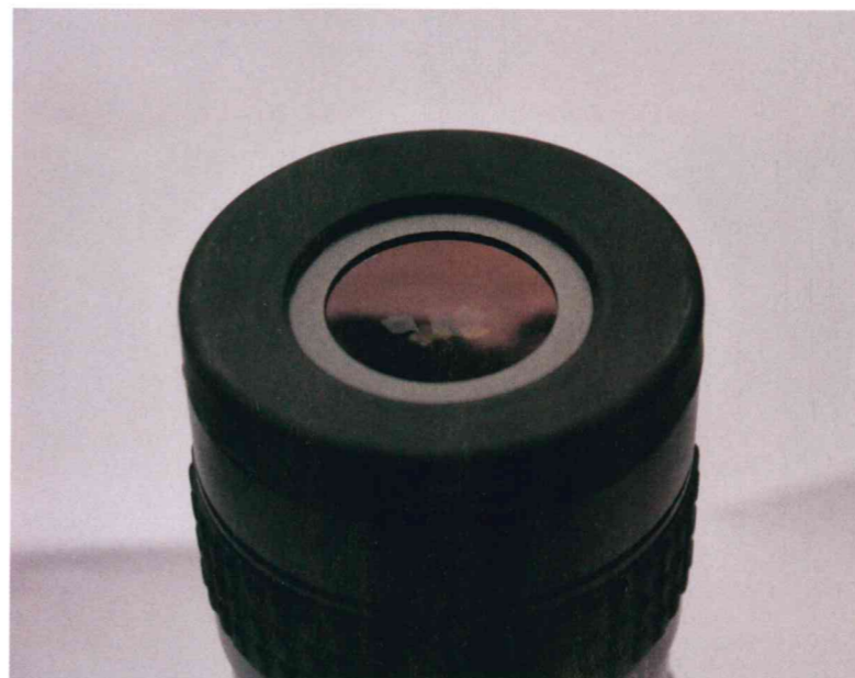
The Baader Hyperion zoom has phantom coatings to increase contrast and minimise internal reflections.
