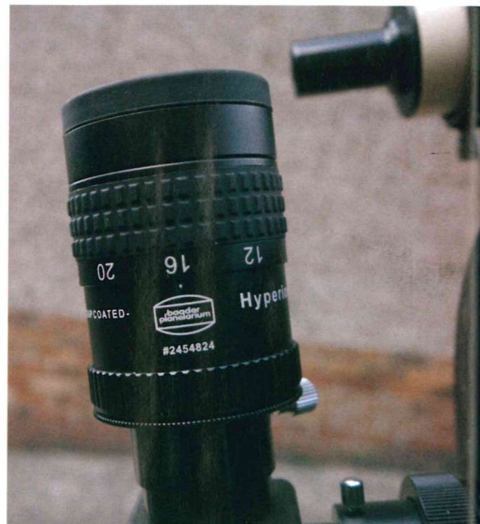
The Baader zoom has click stops to increase or decrease magnification.
