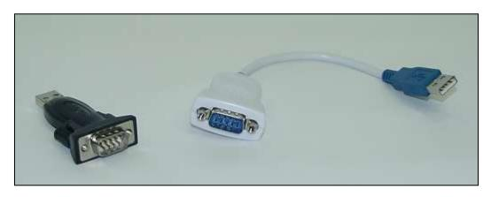
Figure 2-4. USB-to-Serial Converters using the FTDI Chipset.
