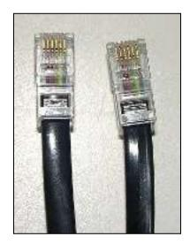
Figure 2-3. Close up of Reverse Cable Plugs – note each end is wired identically.
