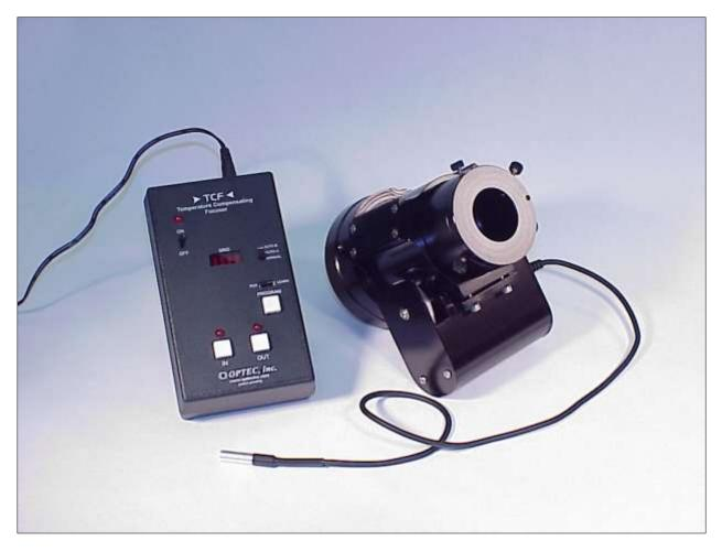
Figure 1-4. Original TCF-S Focuser with Hand Control.
