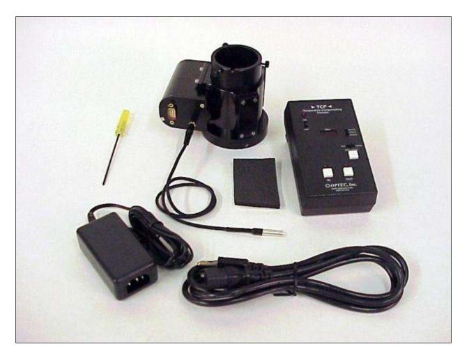
Figure 2-2. Items Included with TCF-S focuser. Focuser body, hand controller, temperature probe, adhesive thermal foam, international switching power supply and U.S. wall plug, and ball driver.
