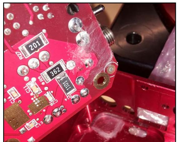
Figure right: Detail view of the strain relief of the very heavy spiral cable of the hand control of the mount at the connector of the RA motor cable
