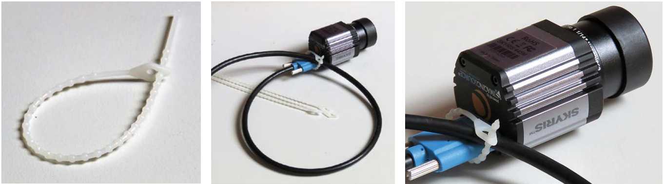
Fig. 01: Cable tie that can be opened again (knotted strap). Fig. 02 and 03: Cable loop directly at the USB 3.0 connector of a Skyris camera with knotted strap for securing
