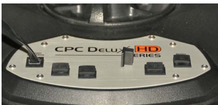
Protective caps prevent that moisture can get in unoccupied sockets, or cables are connected incorrectly and cause short-circuit
