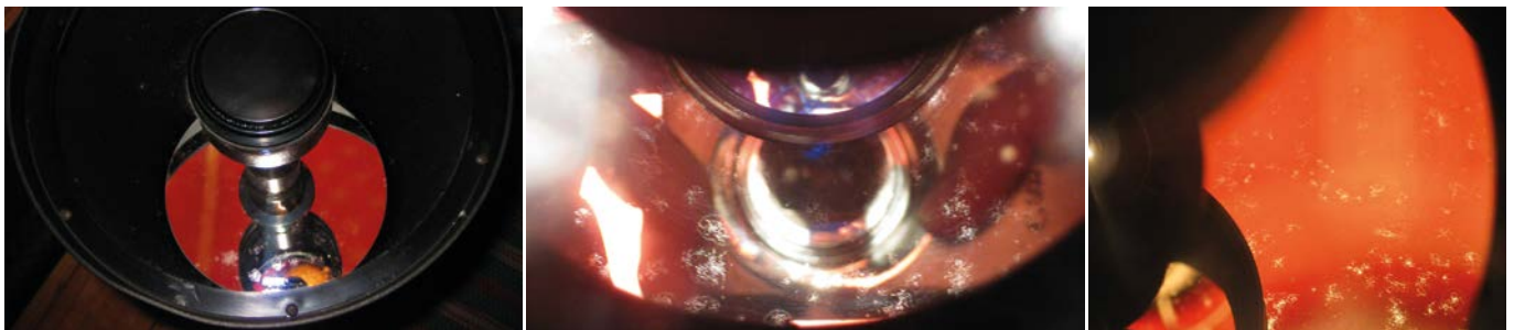
These pictures show the view into a Schmidt-Cassegrain, which was stored for several years in a warm and humid climate by the sea. Even the closed tube of an SC could not provide protection against fungal attack under these conditions.
