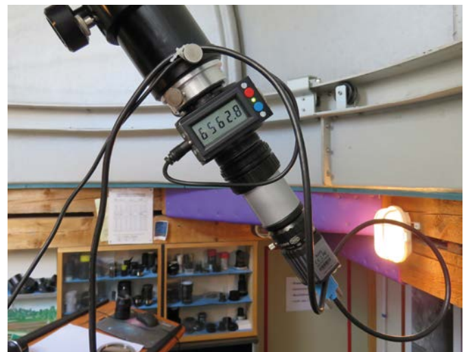
Cable protection on H-alpha filters: Looped, tensioned cable USB 3.0 and power supply, attached to the clamping screw of the eyepiece extension.
