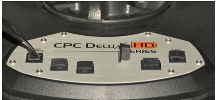
Cover caps prevent moisture from getting into unoccupied sockets or cables from being connected incorrectly and causing short circuits.
