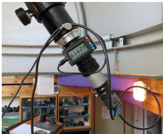
Cable Lock to H-alpha filters: looped, supplied laste steady USB 3.0 cable and power supply, attached to the focuser locking screw.
