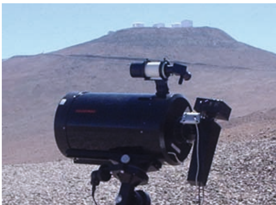
Figure 1: BACHES attached to a Celestron CGE 11" telescope with a Losmandy Equatorial G-11 mount.
