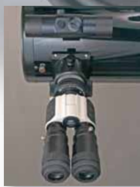
Maxbright-Bino, 8" Celestron-Newton, 5mm Hyperion, Baader Foresight in one Ultrashort-Adapter, 2" Bino Coma Corrector 1.7x, Baader Sky Surfer V Foursight
