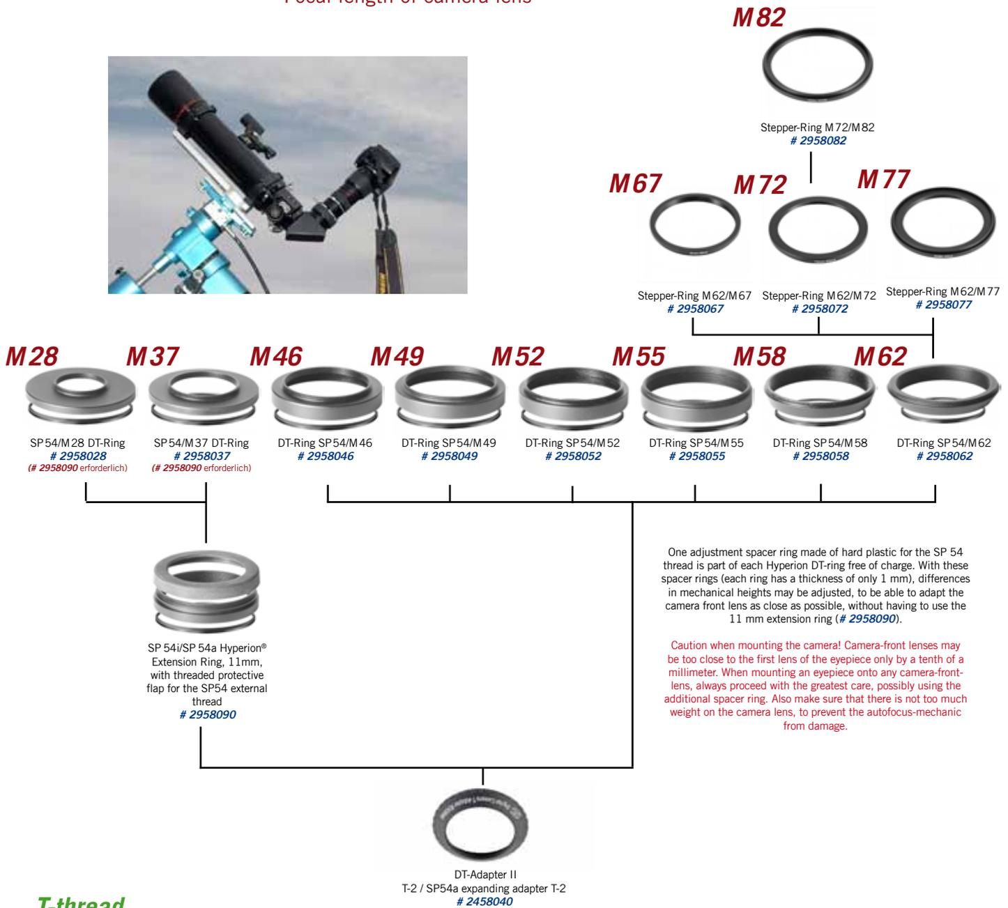
One adjustment spacer ring made of hard plastic for the SP 54 thread is part of each Hyperion DT-ring free of charge. With these spacer rings (each ring has a thickness of only 1 mm), differences in mechanical heights may be adjusted, to be able to adapt the camera front lens as close as possible, without having to use the 11 mm extension ring (# 2958090).
