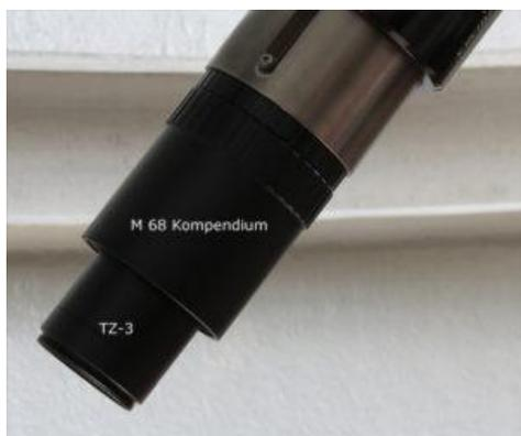
Due to the rather high overall length (the optimum focus position is 250mm behind the last lens center of the [TZ-3](#)), I've mounted the telecentric system inside of an M68 telecompendium.
